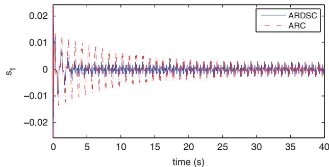
Figure 1. Output tracking errors using ARDSC and ARC, respectively.
